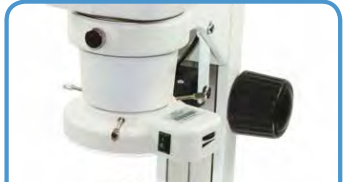
Led ring light with adjustable light intensity.
