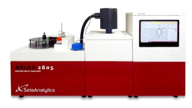
AFIDA is a revolutionary development providing fully automated determination of the Indicated Cetane Number (ICN) of diesel and diesel related fuels.
