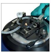
Dip the test flame, flash detection is automatic
