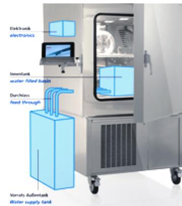
Testing freeze-thaw resistance in a tailor made **test assembly: Memmert temperature test chamber** with water-filled basin inside
